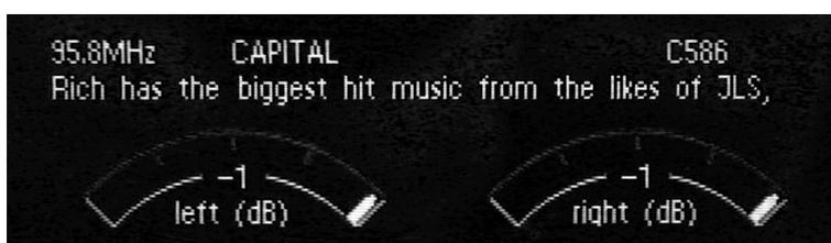
This screen displays the tuner frequency, programme service, programme identification, and radio text in addition to the left and right level of the demodulated received signal.
